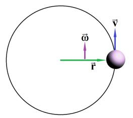
$KE_{Translational} = \frac{1}{2}mv^{2} = \frac{1}{2}m(r\omega)^{2} = \frac{1}{2}mr^{2}\omega^{2}$   $KE_{Rotational} = \frac{1}{2}I\omega^{2}$   $\frac{1}{2}mr^{2}\omega^{2} = \frac{1}{2}I\omega^{2}$   $I = mr^{2}$ Note: This is only valid when all the mass is located at
