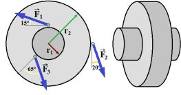
$$\sum \tau = \tau_1 + \tau_2 + \tau_2 = r_1 F_1 \sin 75^\circ - r_2 F_2 \sin 70^\circ + r_1 F_3 \sin 65^\circ$$
