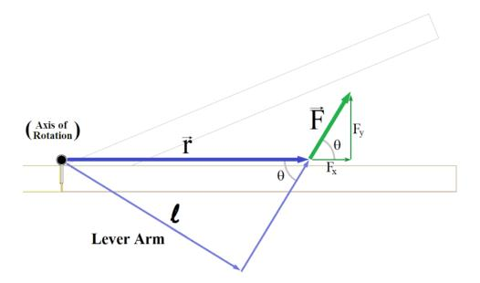
If we apply a force  $\vec{F}$  to an object, we define the vector  $\vec{r}$  to start at the axis of rotation and at the position where the force is applied.  $\theta$  is defined to be the angle between  $\vec{F}$  and  $\vec{r}$ .
