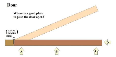
Force A doesn't work very well. A lot of force leads to little movement of the door. Force C is the best option. A little force here is usually enough to open the door. Force B requires more force than C, but not as much as A. Force D doesn't open the door at all.
