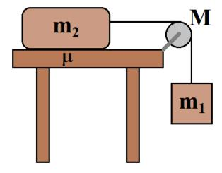
Make 3 force diagrams (one for each object). There are 3 unknowns (2 tensions and acceleration). This means you will need 3 equations, one from each force diagram. Angular acceleration is not another unknown as it is directly related to the acceleration in this problem.
